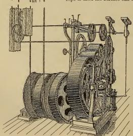
are operated by a tangent-wheel in the casing, which serves as a guard to shift the belt at the extremes of the run of the cage or platform suspended on the drum. The small quadrant seen in front is to move a cord or chain by which the hand movement of the shifting gearing is effected. Fig. 4935 is a view of another of William Sellers and Co.'s winding drums, driven by a train of spur-
